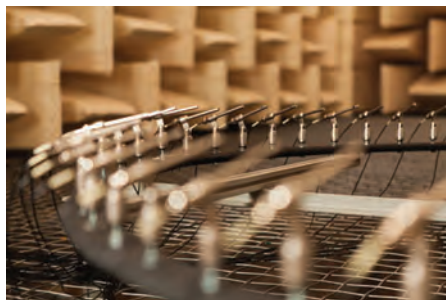
Microphone ring array with intelligent acoustic measurement technology by Fraunhofer
