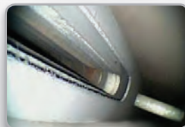
Rotor slot with coil locating dowel
