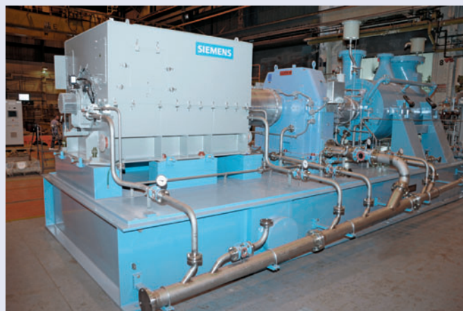
Dresser-Rand Datum centrifugal compressor like the one to be used at the gas processing plant in the Delaware Basin
