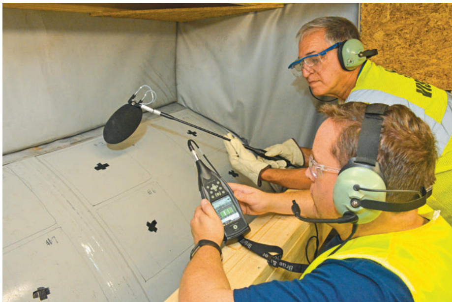
Figure 2. Noise measurement team collecting the sound intensity data inside sealed enclosure on the compressor casing
