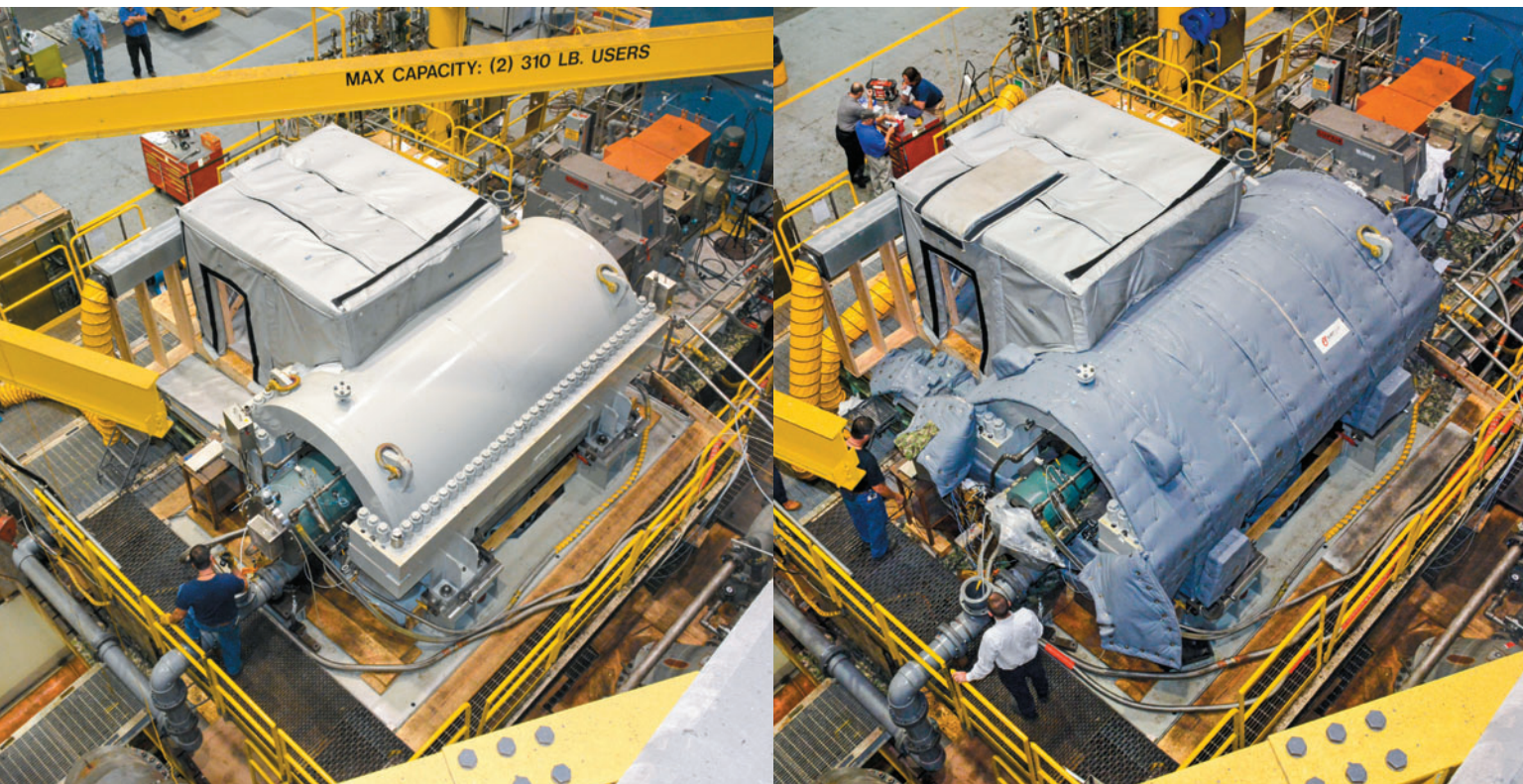
Figure 1. Compressor noise testing with no acoustic blanketing (left) and with acoustic blanketing (right)
