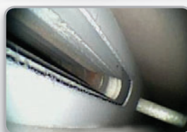
Rotor slot with coil locating dowel
