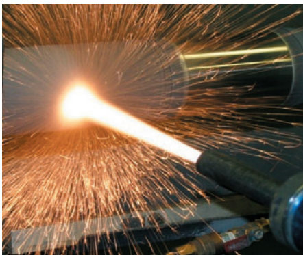
A high velocity oxygen fuel (HVOF) torch applies tungsten carbide to a turbine shaft.
