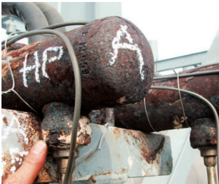
Corrosion found under insulation blankets covering condensate pots
