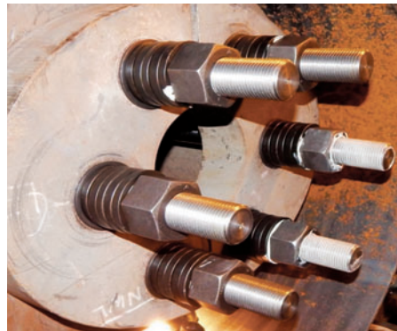
Spring washers are recommended to maintain tension and compression
