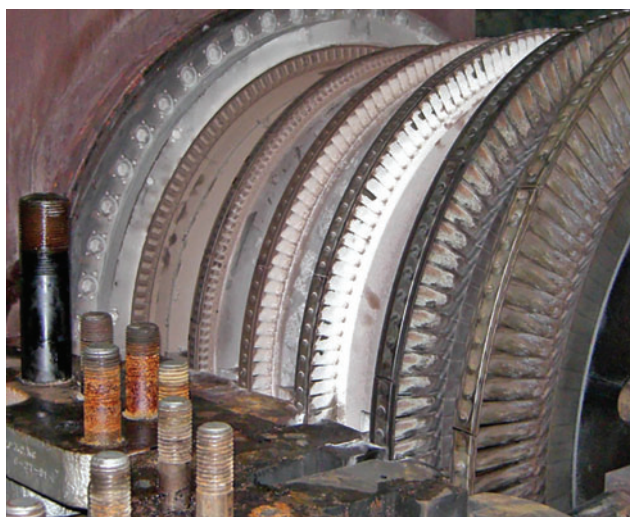
Figure 1. Turbine rotor with mineral deposits.
