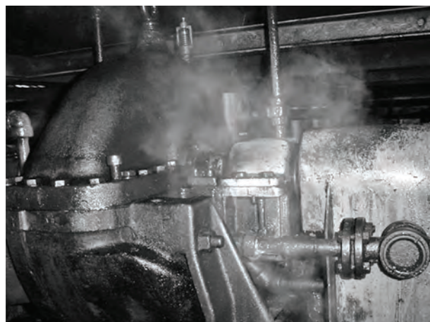
Figure 1: Steam leakage is commonplace from a steam turbine.
