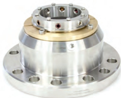
Figure 4: Cartridge-style steam turbine gland incorporating a dry gas seal-based high-temperature mechanical seal
