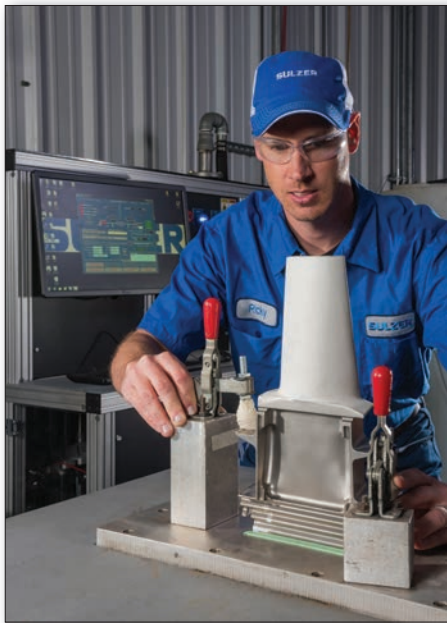
Figure 3: Flow test of 7001 1st stage bucket on high-flow test bench
