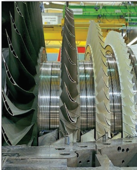
The rotor of a Siemens SGT5-4000F GT during assembly
