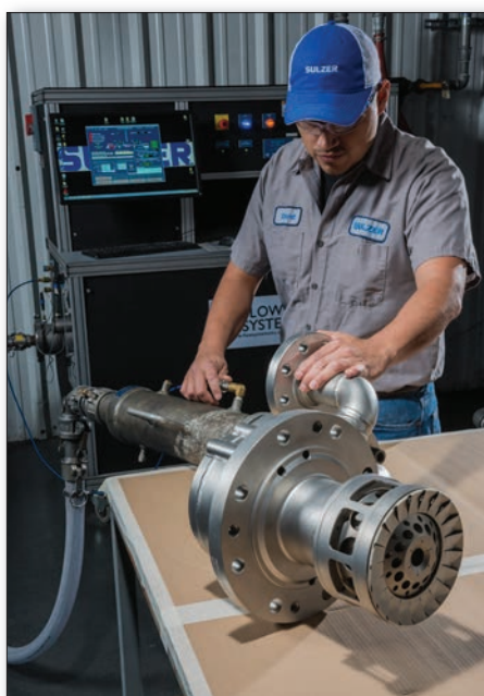
Figure 2: Flow test of 501 DF42 fuel nozzles with steam injection on high-flow test bench
