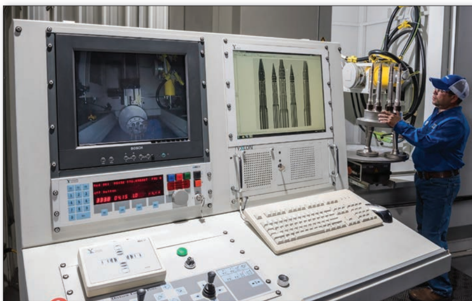
Figure 1: Inspection of 501 FD2 dual fuel support housing in Sulzer's 450 kV, 5-axis digital imaging X-ray booth
