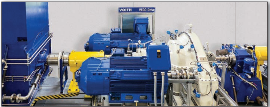
The Voith VECO-Drive steps up input speed and generates a high output speed for compressors or pumps. Since additional power is supplied to the drive train, a smaller main motor can be used for this variable speed drive
