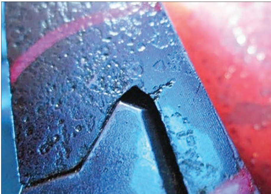
Cracks were found on the last five stages of a 7FA.01 compressor
