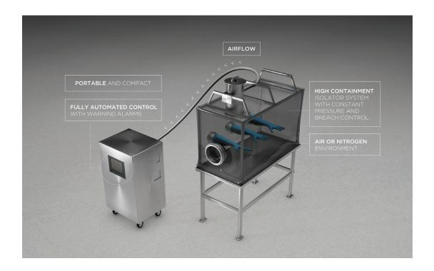
Both oxygen  $(O_2)$  and relative humidity (RH) monitoring is available with the JetVent and when provided with a suitable supply gas and configured with the desired set-points and alarms, the JetVent modifies the atmosphere within the isolator to ensure a maximum  $O_2$  and RH level. This fulfills a common operating requirement of the isolator that cannot be guaranteed in the static form.
