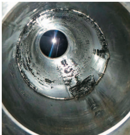
Fitted bolts that seize must be removed by force, which damages the coupling hole
