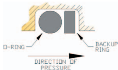
Keep O-rings and back-up rings clean and lubricated before installation
