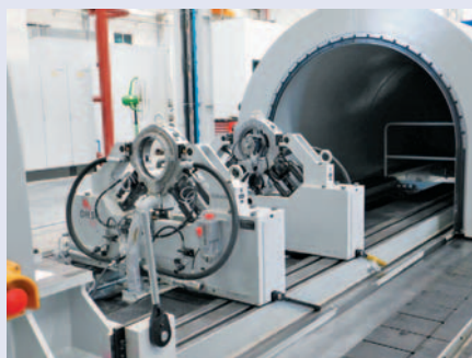
High-speed balancing machine for rotating equipment tests
