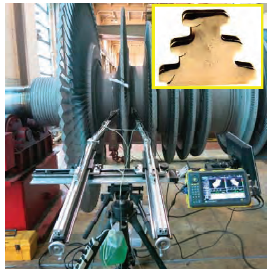
PHASED ARRAY ULTRASONIC TESTING OF ROTOR DOVETAILS & DISKS
