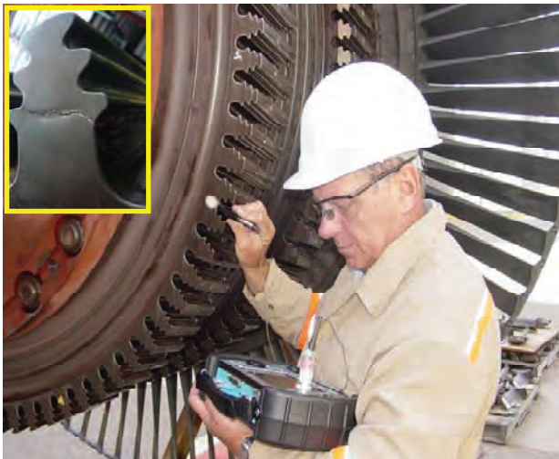
EDDY CURRENT TESTING OF 7FA TURBINE DISK SERRATIONS
