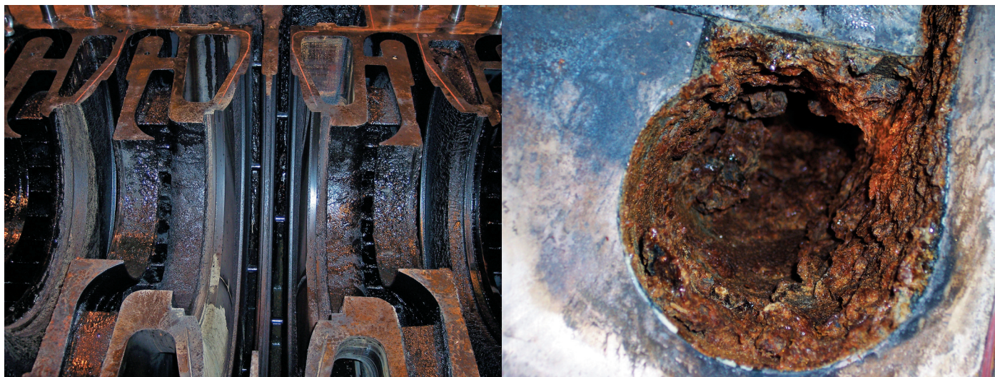
Figure 1. Cracked gas compressor fouling: CGC LP casing after operation (left), and HP casing (right). As a result of fouling, the accumulation of polymers on the internal surfaces adversely affects overall performance. Changes in feedstock or cracking severity can change or shift the dominant fouling mechanism.
