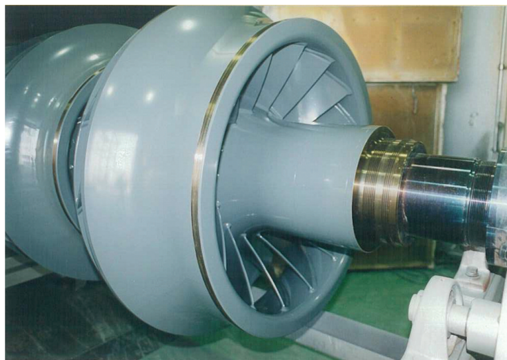
Figure 6. SermaLon coating of internal components
