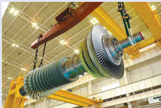
MHPS J-class gas turbine
